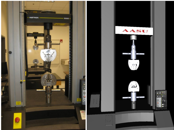
Figure 1. Instron™ 5566 real TTM (left) and 3D model (right).
